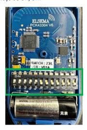
5. Lastly, insert the battery and test the functions.
