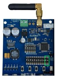
4. Set DIP switches 1-10 in the remote exactly the same as the receiver. Dip switch 11 and 12 should always be Off/Off.
