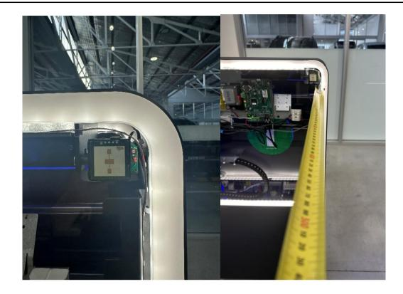
11. Set radar distance to **2000mm** with the cover on using a measuring tape and the red LED indicator light to show that it is detecting customers.
