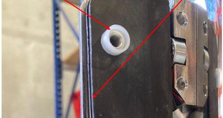
Gently tighten gate arm bracket screws until the plastic spacer flattens up tight to the polycarbonate arm panel. Make sure check that the rubber gasket and plastic spacers are not overlapping each other, and all components are aligned correctly before firmly tightening all gate arm fixings in place.
