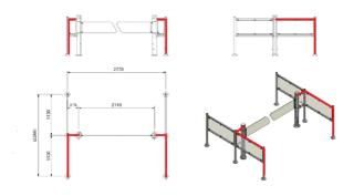
RED LINE REPRESENTS INTERNAL PEC SENSORE ROUTING
