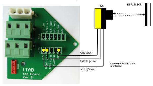
In a photocell eye system, the gate opens when an object breaks the infrared beam, and closes automatically after a set period, once the object has been cleared from the beam – this period of time is adjustable by adjusting the right hand (Master) gate bollard Delay/SCO potentiometer on controller PCB.
