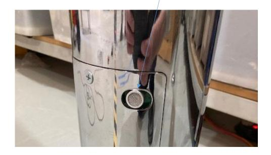
8. Fit new type radar sensor cover-strip (if supplied) before CSS commissioning commencement.
