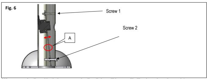
(When properly aligned both the green and yellow lights will be steadily illuminated continuously)
