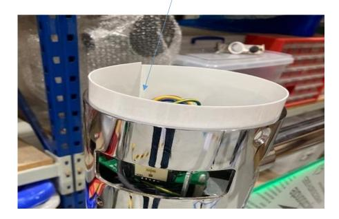
(Radar cover slides in & out without fixings cover to join to the side away from gate bollard cut out)
