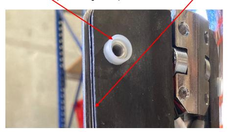
Gently tighten gate arm bracket screws until the plastic spacer flattens up tight to the polycarbonate arm panel. Make sure check that the rubber gasket and plastic spacers are not overlapping each other, and all components are aligned correctly before firmly tightening all gate arm fixings in place.
