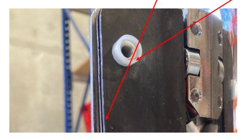
Gently tighten gate arm bracket screws until the plastic spacer flattens up tight to the polycarbonate arm panel. Make sure check that the rubber gasket and plastic spacers are not overlapping each other, and all components are aligned correctly before firmly tightening (all 12 Allen bolts with preapplied to screws) gate arm fixings plate into place.
