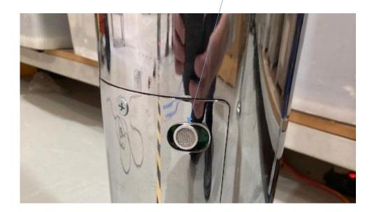
9. Fit new type radar sensor cover-strip (if supplied) before CSS commissioning commencement.
