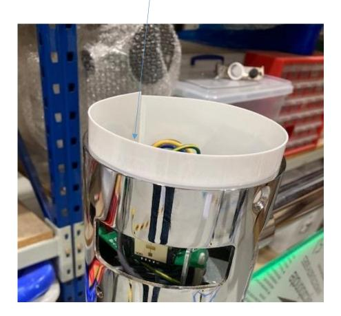
(Radar cover slides in & out without fixings cover to join to the side away from gate bollard cut out)
