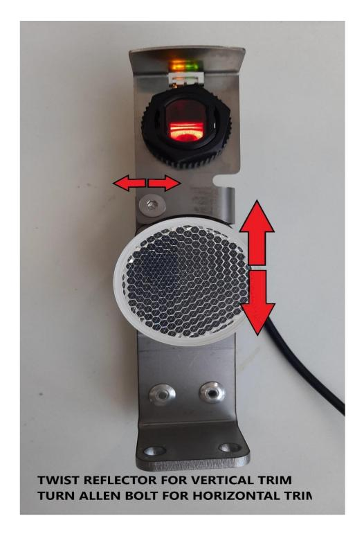
Break the beam and test gate operation: **important:** when PEC is set (trimmed) correctly, **both** the yellow & green lights will be **steadily** on at the same time – see image above.
