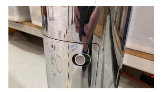
9. Fit new type radar sensor cover-strip (if supplied) before CSS commissioning
