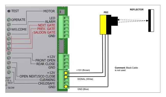
This PEC triggers the rear gate couple and is mounted into the front gate bollards.
