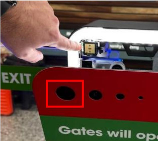
**NOTE!** If the out cut is slightly blocked by the magnetic sticker, it will limit the coverage of the safety radar trigger zone.
