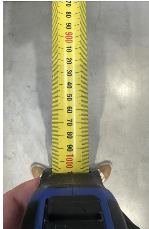
10. Set radar distance to 1M using a measuring tape and the red LED indicator light to show that it is detecting customers.
