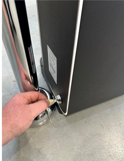
2. Open SigmaGates using the remote and the turn gate off by turning the key to the vertical position or cut the power to the gate.
