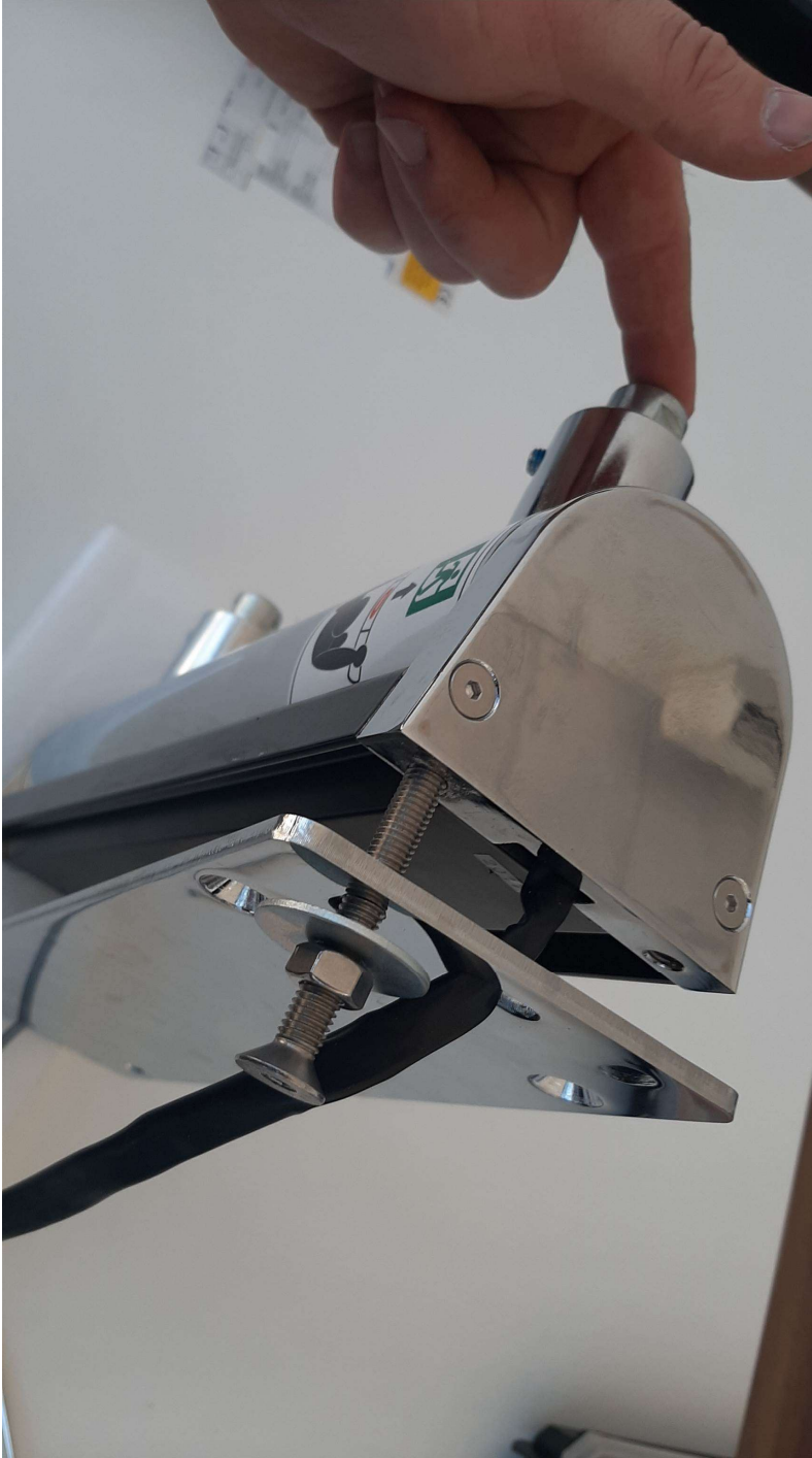
(DR6) Below: image of ACC drive assembly with backing plate and fixings inserted.
