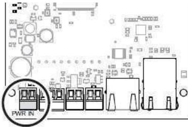
1 Disconnect the 12V power supply cable to cut the power.
