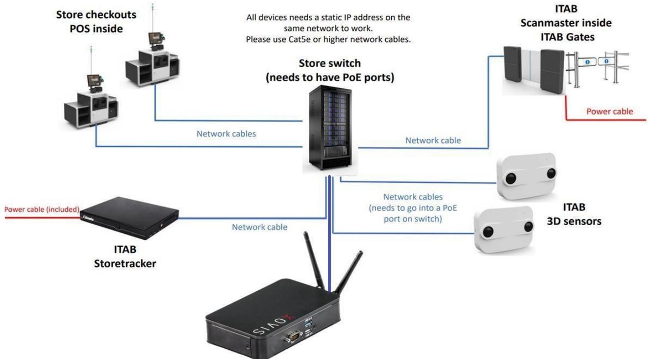
Note: Store checkouts and POS systems are already connected to the store switch and it is not necessary/required to run additional patch leads to the checkouts.
