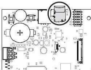
2 Put the Micro SD card for specific gate to the GateMaster board.
