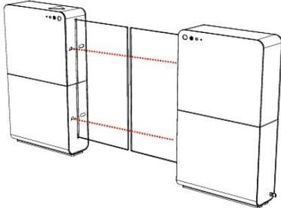
Make sure the two photoelectric cells (PEC) are pointing at the reflectors on the other gate.
