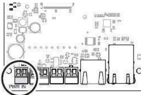
3 Connect the 12V power supply cable.
