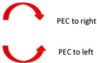
To adjust the PEC, use Allen key 2.5 mm.
