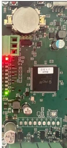
4 The ScanMaster board will now go through an initialising process (allow 90 seconds). Once initialising is complete the LEDs will blink green on LED number 1 and be solid red on LED number 10. LED number 5 will blink orange once when the gate receives a message from POS.
