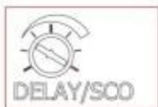
**DELAY:** This sets the amount of time the gates will stay open after a customer has left through the gates and broke the PEC sensor beam. Range 0-8 seconds. Note: This timer will over ride the secure timer.
