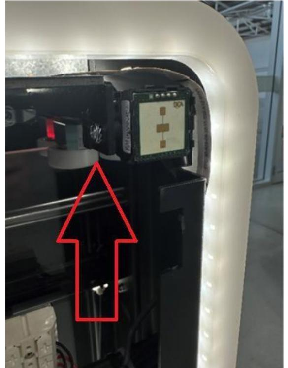
Remove the screw and washer from the bracket and discard the bracket supplied. Use the bracket screw to mount the customer facing radar to the bracket in the corner of the SigmaGate
