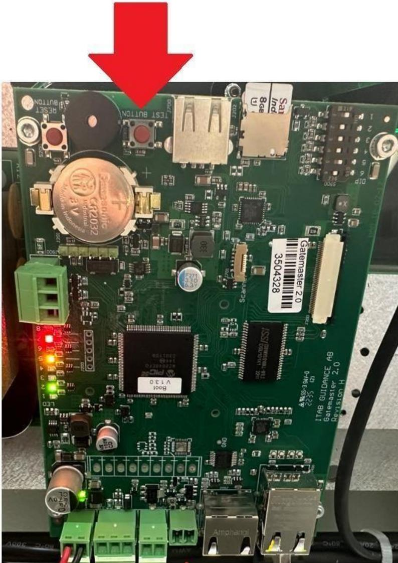
Use the test button on the ScanMaster/GateMaster to trigger the gate. This will send an open gate signal to help check the timing of the gate. Please note that this will only trigger the gate and start the Secure timer until the PEC sensor is broken.
