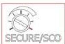
**SECURE:** This timer will keep the gates open until the customer has passed through in the gates. Once the customers pass through the gates this timer is gets override by the DELAY timer. Range 0-30 seconds
