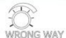
**WRONG WAY:** This timer is used to detect movement through the gates in the wrong direction. Please set to full right to avoid picking up a customers swinging arm. Range 0.1-2 seconds
