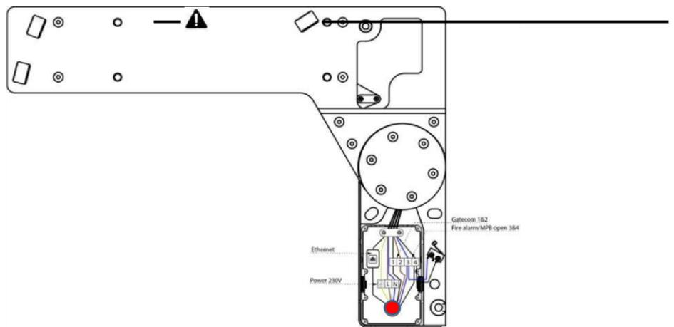
The data cable is to be routed directly from the store switch/coms cabinet to the ScanMaster board directly with no breaks in the cable. Open circular plate and run data cable through the MPB bracket, ensuring that the data cable is looped around the metal cable protector then plugged directly to the ScanMaster board.
